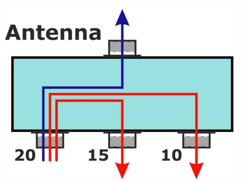
*Leakage from transmit port - 20, to receive ports - 15 and 10!*
