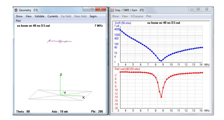
Removing D3 moves resonance up to 8.5 MHz – progress!
