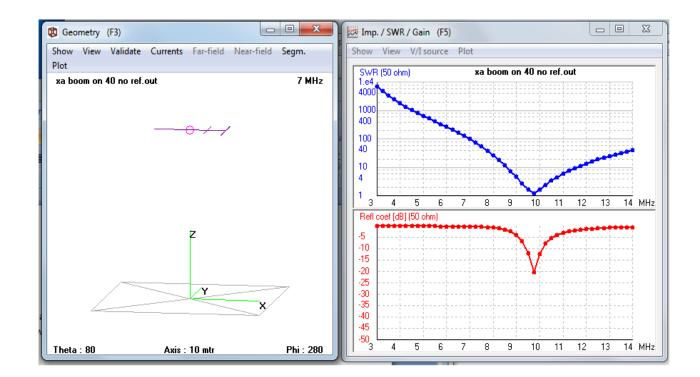
Removing reflector has greatest effect – resonance moved to 9.75 MHz!
