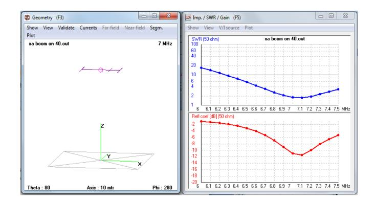
Note XA boom is resonant on 40m – Would make a nice dipole!!
