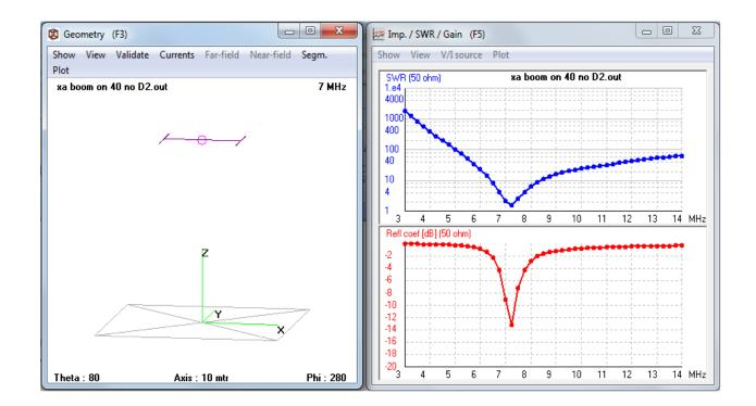
Removing D2 has very little effect – Reflector and D3 still provide loading
