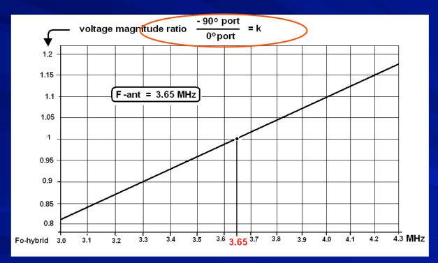
With unequal resistive loads  $(Z_2,Z_3)$  we can obtain k=1 by shifting the design frequency of the hybrid
