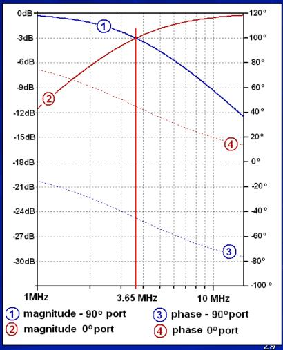
k = ratio of voltage magnitude at port 2 vs. voltage magnitude at port 3
