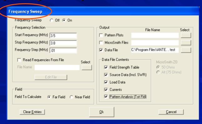
The EZNEC modeling software creates a .txt file with all data in selected frequency steps
