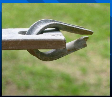
The proper thimble is known as a "heavy duty" thimble, identifiable by its distinctive shape.
