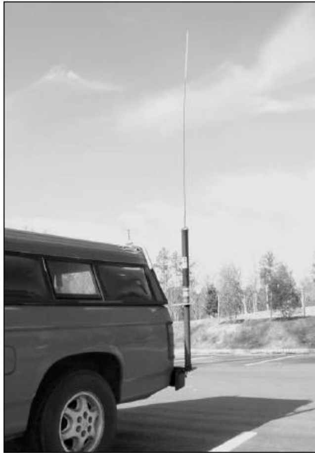
Fig 23—The completed Screwdriver antenna mounted on KO4TV's truck rear bumper. (Photo courtesy of Gary Pearce, KN4AQ.)
