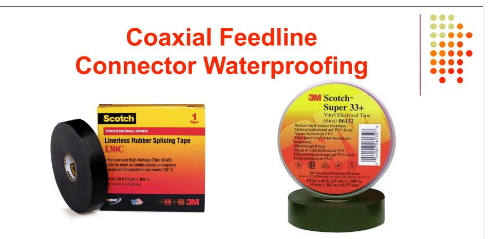
Cover the connectors with two 50% overlapped layers of Scotch 130C stretched to 50% of its original width
