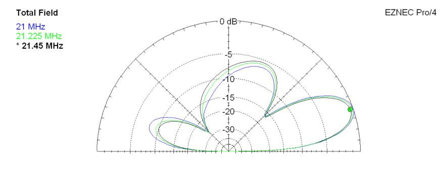
Elevation Plot Azimuth Angle 0.0 deg. Outer Ring 11.94 dBi
