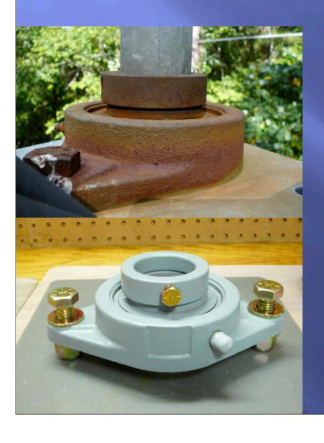
They are not weather-rated and rust quickly, allen set screw on the collar is often a problem, and the bearing requires lubrication
