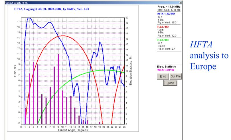
At 3°, K6TA's hill gives him 20 dB over a dipole at 50' on flat ground! At 9° the advantage narrows to 10 dB. 37
