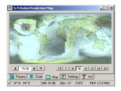
*HamCAP* shows SNR on a small rectangular map for current solar conditions. This is elegant and more intuitive. But it is still a "snapshot" for only one band/one UTC. And hams still aren't really comfortable with SNR in a 1-Hz bandwidth.
