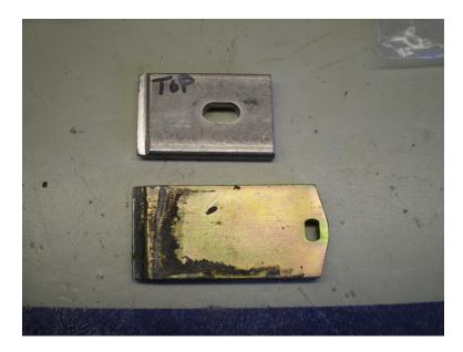
Note that the wedges have a top and bottom. If you slide the wedge into the bell housing groves – you can quickly figure out which side is the top. They really will only engage one way. If you put it in upsidedown, your brake is not going to engage very well.
