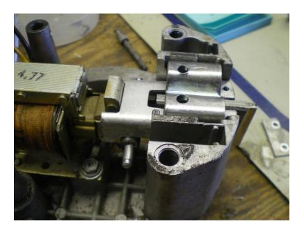
The two holes that are now on top of the retainer assembly each need a spring in them — which helps push the locking mechanism down when the brake is engaged. You can see them here:
