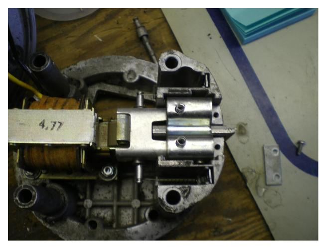
The final step is to install the two springs on each side of the rod that goes through the solenoid flange. These are held in place with flat pieces of metal that slide down into a channel. You can clearly see the spring on the bottom side of the rod in the above photo.
